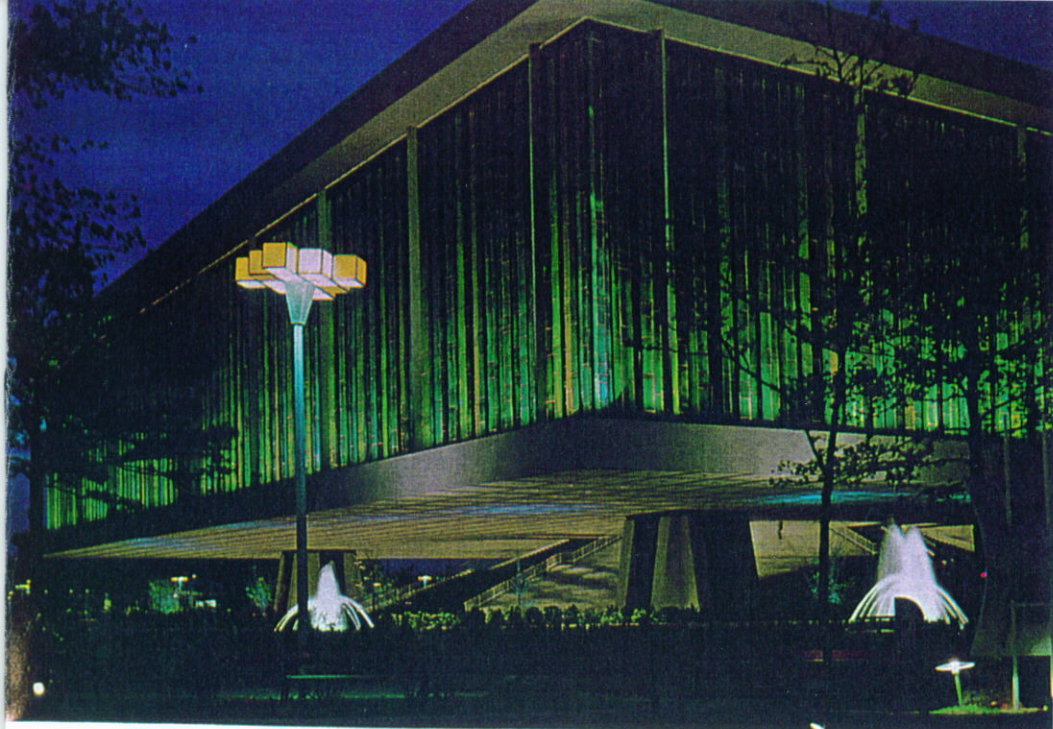
LIGHTING combines with fountains and colored exterior wall panels to give shape and design to the U. S. Pavilion. Basic lighting is with recessed PAR reflector lamps.
