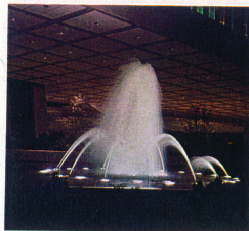
LIGHTING combines with fountains and colored exterior wall panels to give shape and design to the U. S. Pavilion. Basic lighting is with recessed PAR reflector lamps.
