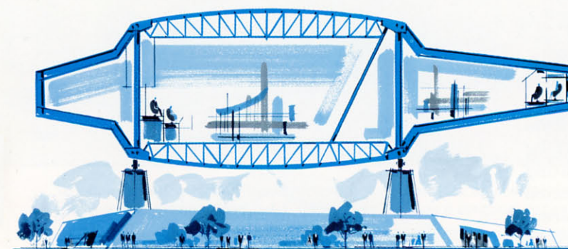
Cutaway sketch of the structure at its midpoint shows how the ride passes through the "long" U-frames; mechanical equipment is housed in the "short" U-frames.
