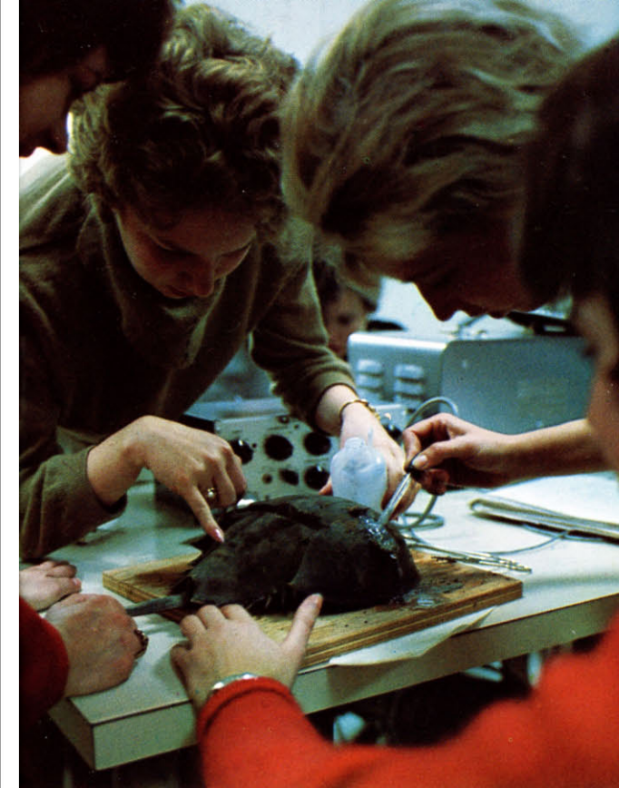
Forty science demonstrators, all of them college girls, dissect a horseshoe crab (above) to obtain its optic nerve. The nerve is attached to an oscilloscope (right), which transfers the impulses traveling the nerve into visible signals on the oscilloscope tube. The experiment is performed in the Methods of Science area of the Science Pavilion.
