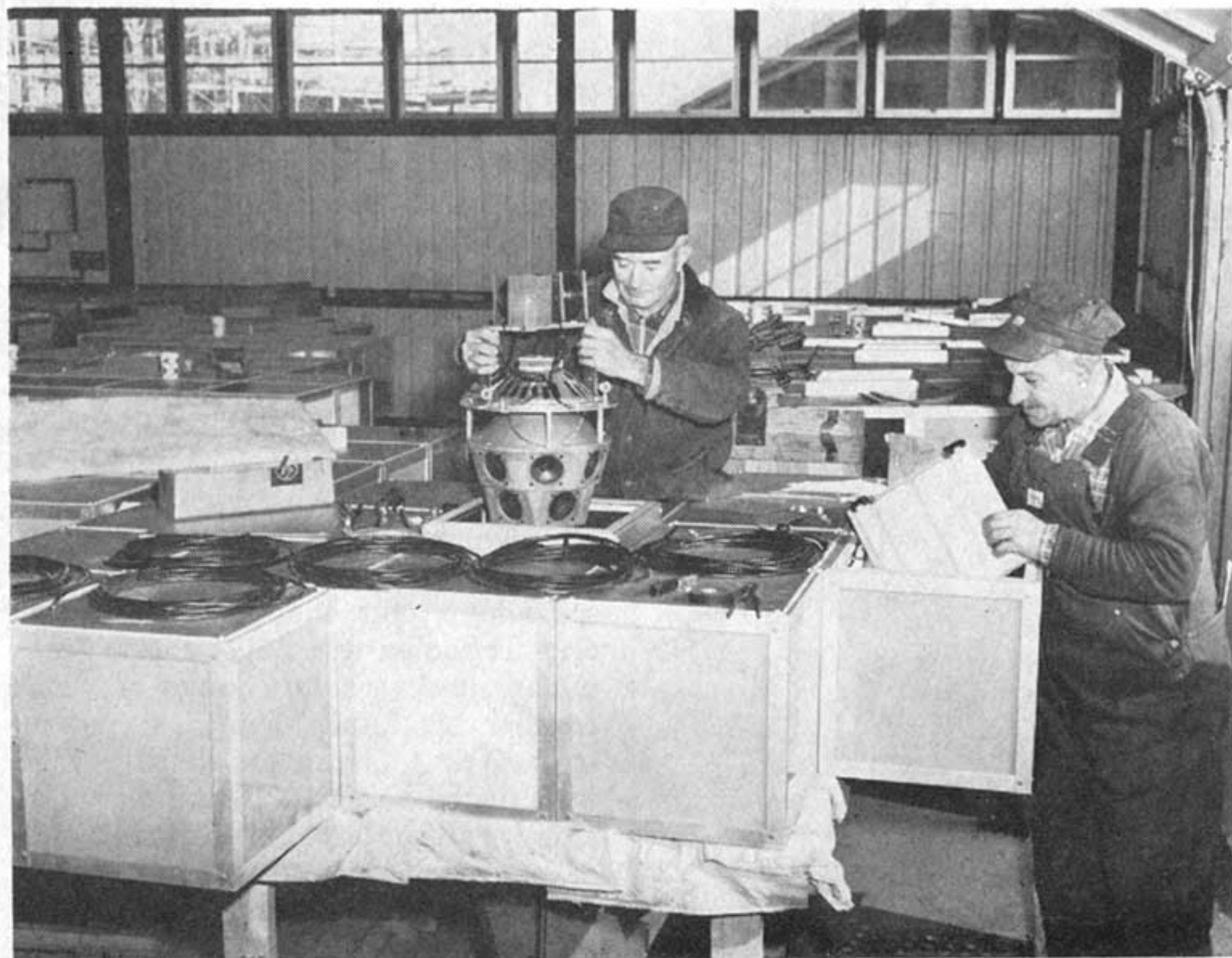
CLUSTER OF SPEAKERS are being installed by worker at center; at right a worker seats a square fluorescent lamp at bottom of the luminaire's translucent cube.
