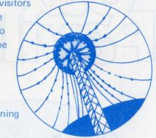
The canopy weighs 12 tons and is large enough to cover two football fields. It is suspended from a 145-foot steel mast, which is tilted at an 8½° angle to compensate for the unequal weights of the roof structure on either side of it.
